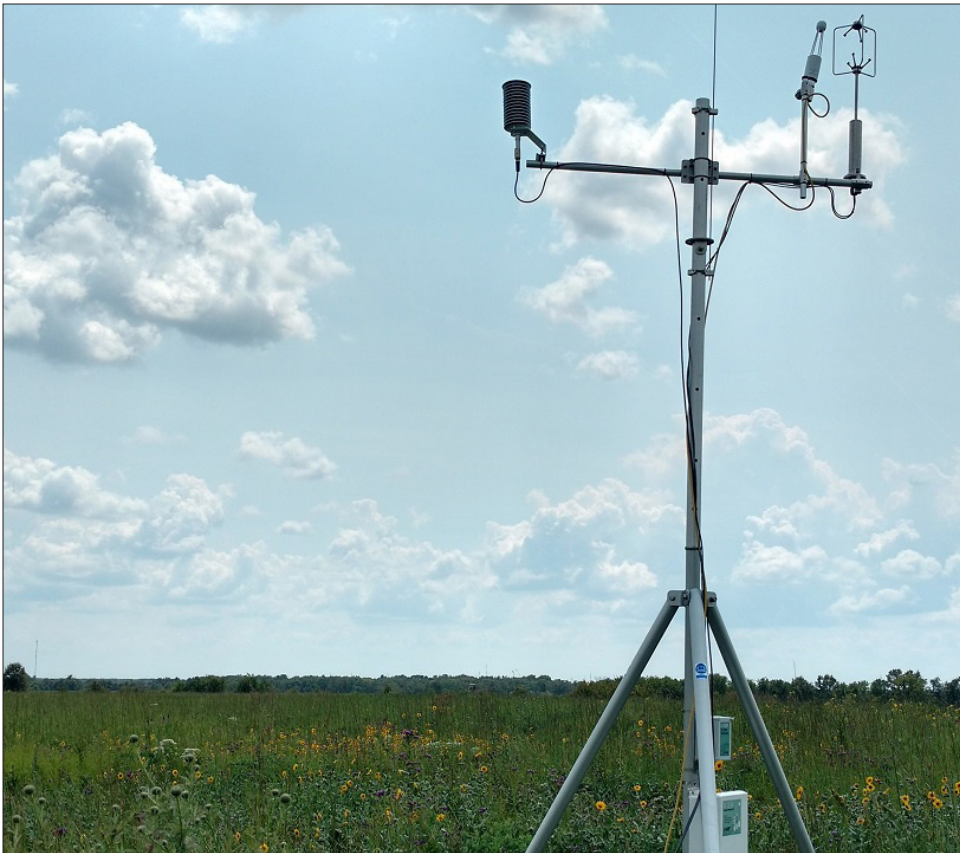
AN EDDY covariance tower, a tool which measures the breathing capacity of an ecosystem, sits in Tucker Prairie, Missouri's largest remaining virgin tall-grass prairie. Photo by Jeffery Wood
